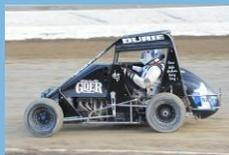
**Minisprints:** Running a midget-sized chassis with a 1400cc engine and moderate wing, Minisprints are another class that is proving its worth as a stepping stone, while still providing the benefits of a National class. Currently raced only in the North Island.
