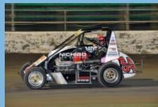
**TQ Midgets:** A “Three Quarter” Midget, TQ's are a pocket rocket version of their larger siblings, running a Motorcycle engine and providing an excellent introduction into the world of Open Wheel racing.
